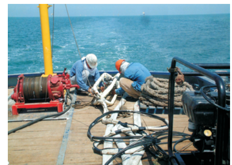
MASW-equipment (air gun and hydrophone chain)
